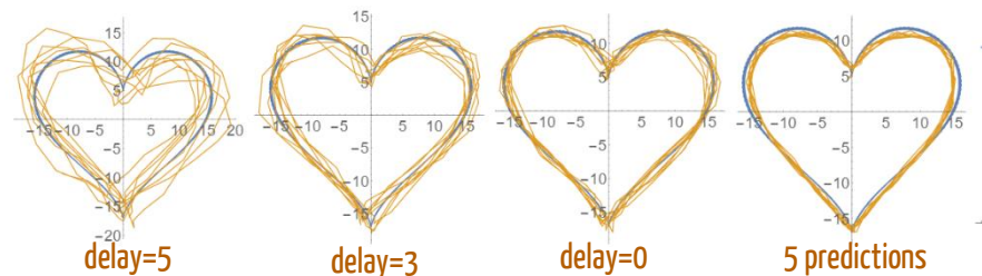
Example: Trajectory tracking with double integrator dynamics
