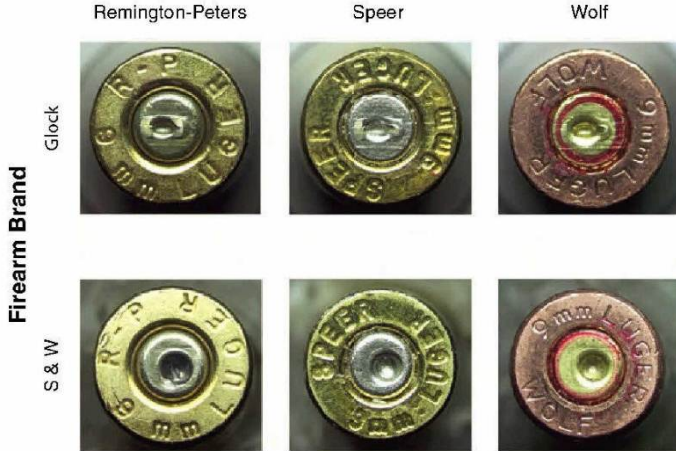
FIGURE 2-2 Breech face markings and firing pin impressions for three ammunition types and two firearm brands.
